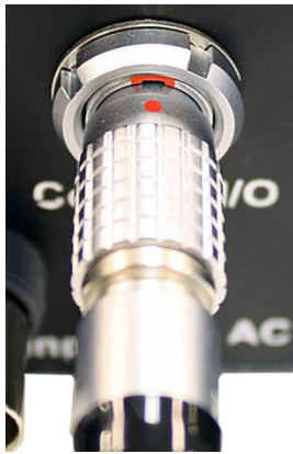
Figure 4: Properly Seated Control Cable.
