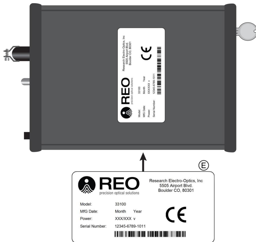
Figure 2: Power Supply Label Placement Diagram
