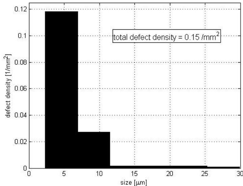
Figure 3. Defect size distribution of one of the Set #2 optics ( $\text{HfO}_2/\text{SiO}_2$  AR).
