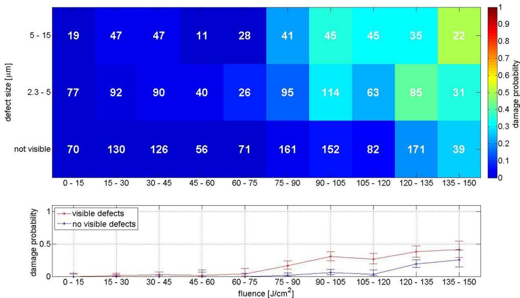
Figure 5. Damage probability map of Set #2 optics (HfO<sub>2</sub>/SiO<sub>2</sub> ARs) as a function of fluence and defect size.
