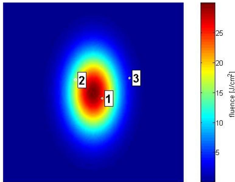
Figure 8. Beam intensity and location of defects for sample damage calculation. The color encodes the local fluence, with a maximum at  $30 \text{ J/cm}^2$ .
