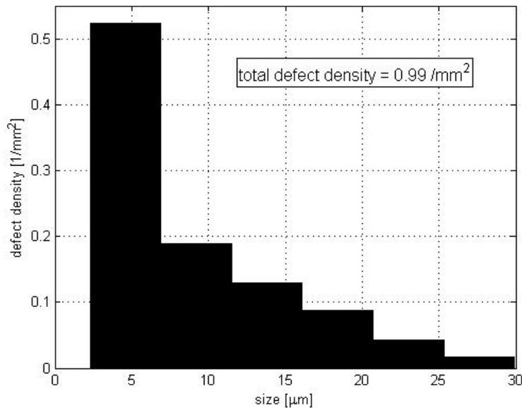
Figure 2. Defect size distribution of one of the Set #1 optics ( $\text{HfO}_2/\text{SiO}_2$  HR).
