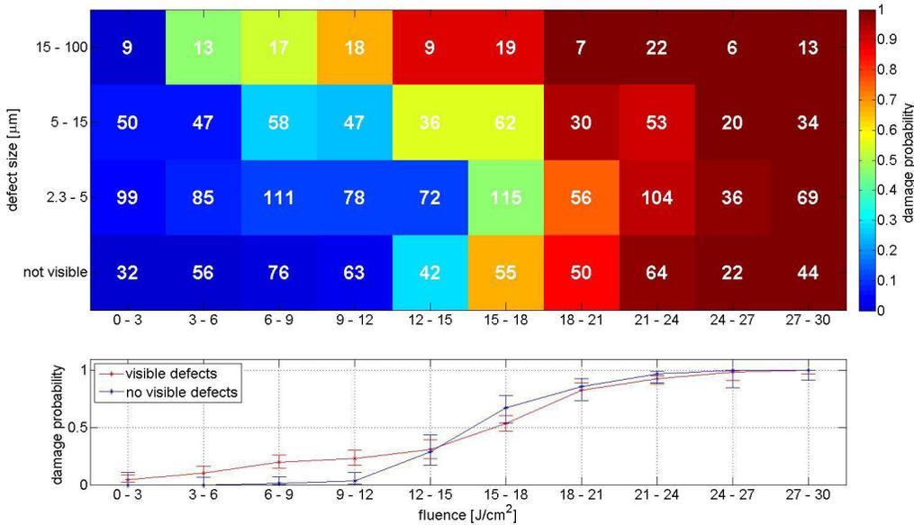
Figure 6. Damage probability map of Set #3 optics (Nb<sub>2</sub>O<sub>5</sub>/SiO<sub>2</sub> HRs) as a function of fluence and defect size.
