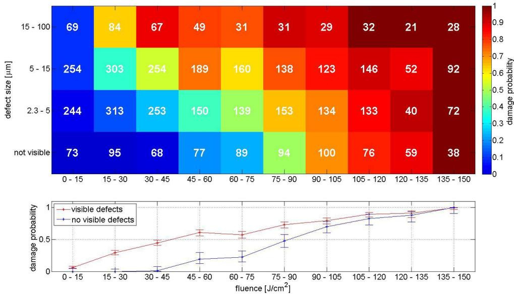
Figure 4. Damage probability map of Set #1 optics (HfO<sub>2</sub>/SiO<sub>2</sub> HRs) as a function of fluence and defect size. The color scale encodes probability, and the number in each block is the number of sites tested at that fluence and size.
