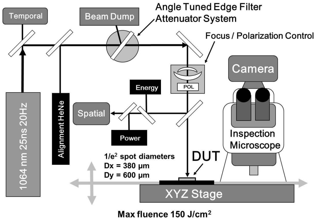
Figure 1. Schematic diagram of laser damage test system.
