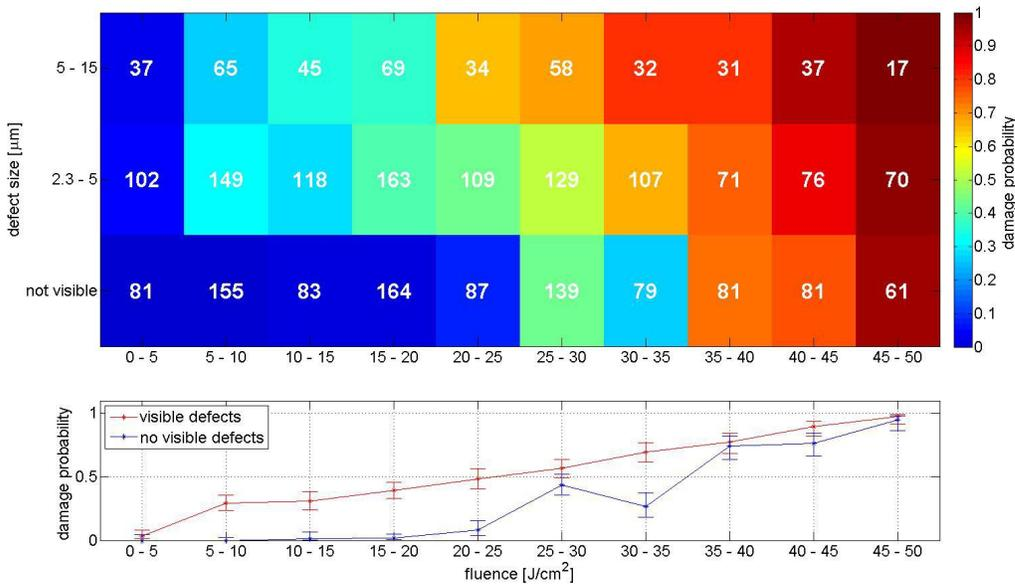
Figure 7. Damage probability map of Set #4 optics (Nb<sub>2</sub>O<sub>5</sub>/SiO<sub>2</sub> ARs) as a function of fluence and defect size.
